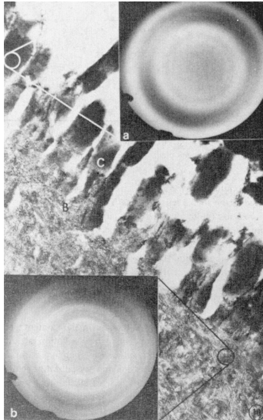
FIGURE 2.15 Transmission electron micrograph of well-mineralized bone (b) juxtaposed to the glass-ceramic (c) which fractured during sectioning. \times 51,500 . Insert a is the diffraction pattern from ceramic area and b is from bone area. (From Beckham C.A., Greenlee T.K. Jr, and Crebo A.R. 1971. Calc. Tiss. Res. 8: 165–171. With permission.)
